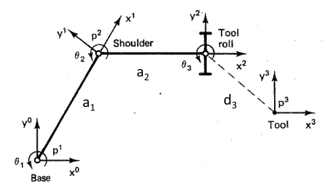
Kinematic parameters from DH algorithm:
