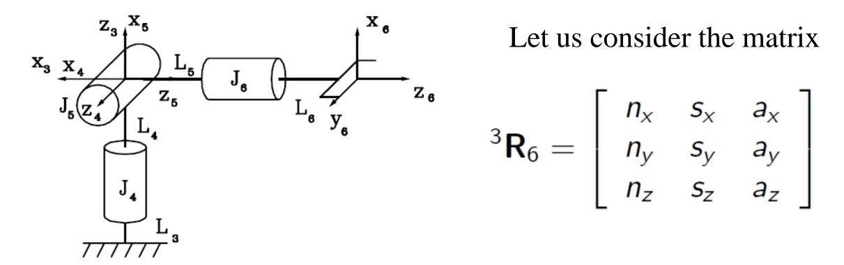
From the direct kinematic equations one obtains
