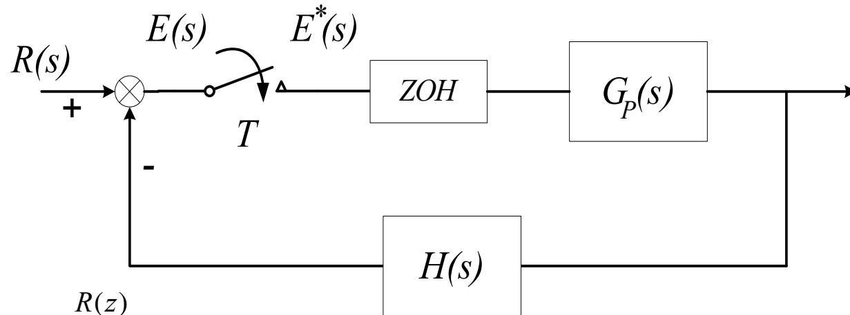
$$\begin{aligned} E(z) &= \frac{R(z)}{1 + Z[ZOH \cdot G_p \cdot H]} \\ &= \frac{R(z)}{1 + (1 - z^{-1})Z \left[ \frac{G_p(s) \cdot H(s)}{s} \right]} \\ &= \frac{R(z)}{1 + GH(z)} \end{aligned}$$
