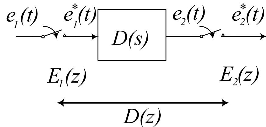
$$D(z) = \frac{b_0 + b_1 z^{-1} + \dots + b_m z^{-m}}{a_0 + a_1 z^{-1} + \dots + a_n z^{-n}}$$
